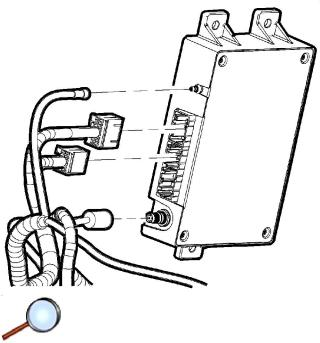
3. Disconnect the electrical connectors, the GPS antenna, and the cellular coax cable.
